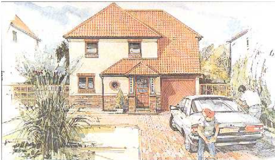
Houses that exploit solar energy do not need overlarge windows on the south side but, like the north face of this house, are designed to reduce heat losses on the north. They look much like other houses but have a market advantage.
