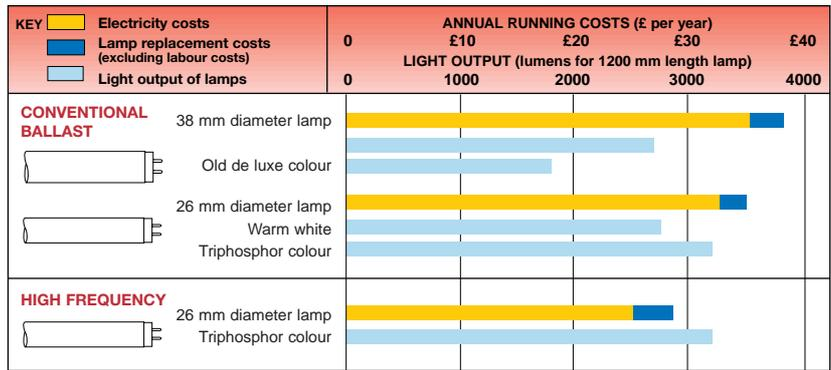
Note: figures for 1200 mm length lamp **Figure 2 Comparison of running costs for different fluorescent lamps**
