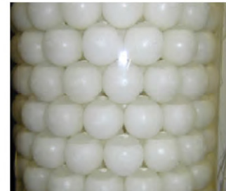
(vi) Fixed bed arrangement with PCM balls
