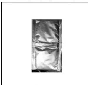
(x) PCM in aluminium pouches
