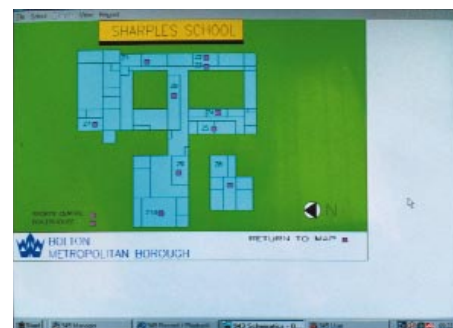
Figure 13 Computer interface for the energy management system – showing heating zones at Sharples School
